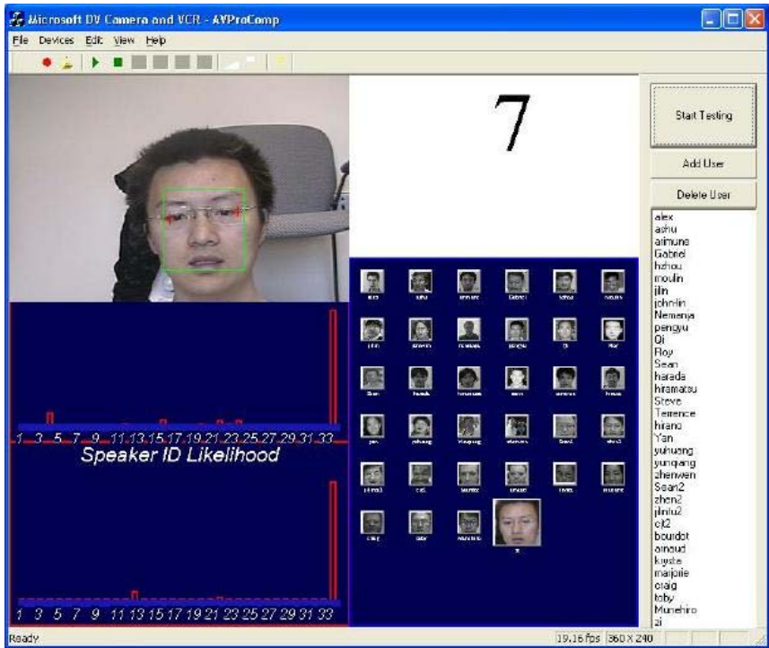
Fig. 16.2. A computer access control system using both face and speaker recognition.
